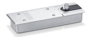
Floor spring for single leaf single and double-action doors of up to 1100 mm leaf width with adjustable closing force EN 1-4 and with optional hold-open function
